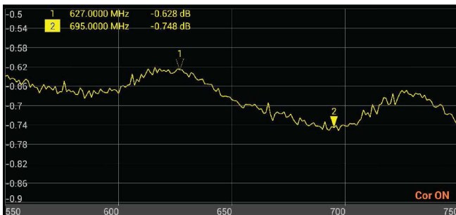
Figure 11 Interpreting Cable Loss Measurement
