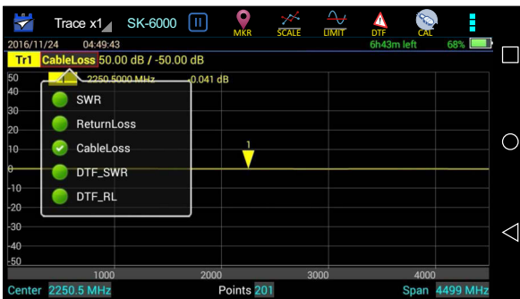
Figure 10 Selecting Cable Loss Measurement
