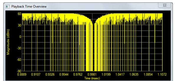
Apply ramp functions to beginning and end of waveform segments to minimize frequency splatter.
